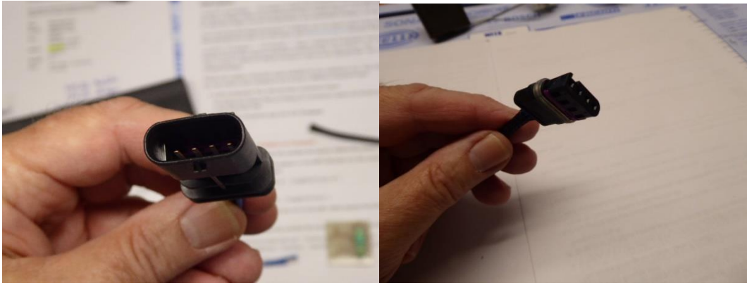
Fig. 9 Use of original BMW connectors so they fit well on the existing connectors.
