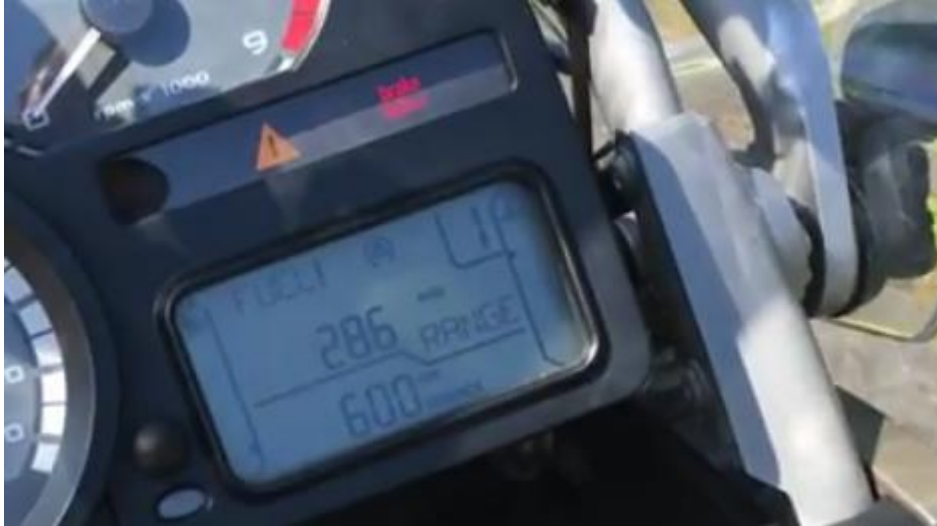
Fig. 1 The display with the annoying yellow sign is due to a defective foil sensor.
