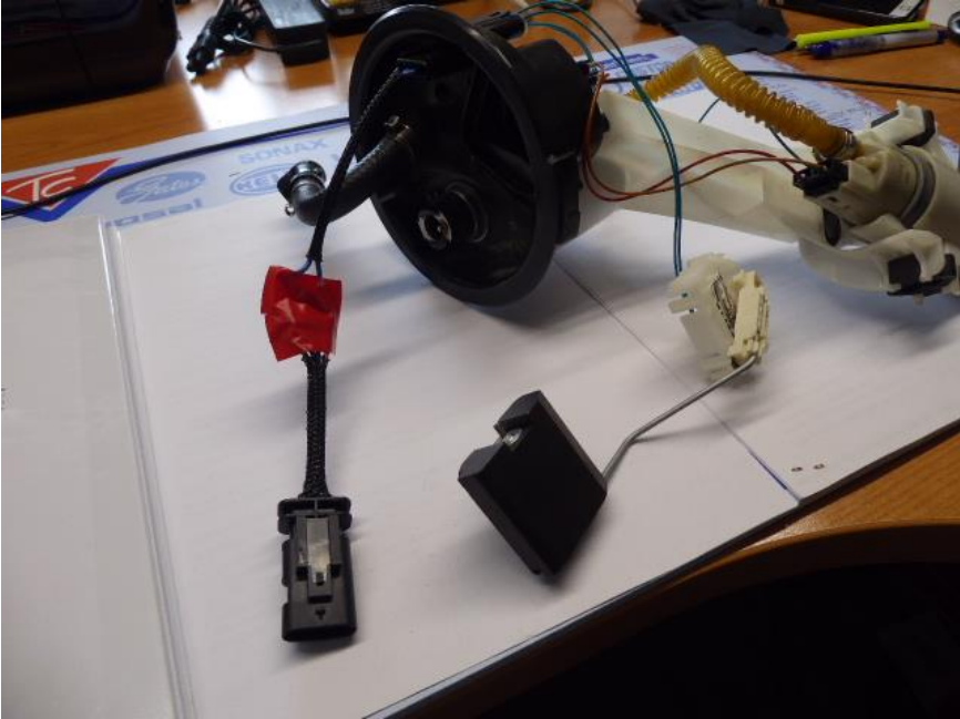
Fig. 3 Prototype of the Float Control on the workbench connected to the tank unit. On this picture you can already see how the Float Control and the wires of the original BMW float should be connected to the fuel pump unit. So, the new float is connected to the connector where previously the connector of the foil sensor was inserted.
